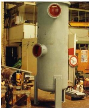
Coatings with VP 10-017 for air coolers, tanks and other big surfaces. VP 10-017-coatings as surface protection and protection against corrosion do offer a very smooth, flexible and wear resistant surface. VP 10-017 is temperature resistant up to 100 °C and offers a very high chemical resistance.
