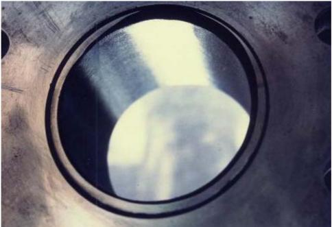
Blocking valves have been reconstructed by using Ceramium. Responsible was serious wear and tear on the steel alloy caused by the clay loam.
