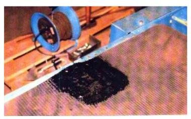
A conveying belt of a compost filling plant showed a 120 mm x 130 mm long triangle fracture at the corner. After cleaning and degreasing with MM-Degreaser Z an application of MM-Elastomer 95 with Hardener EL95 was done. Afterwards the conveying belt was put into action again with a tensile stress of 5 bar.
