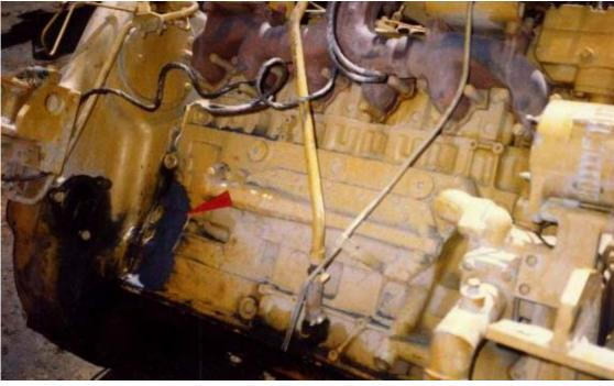
Repair of a hair crack at a main engine block of a bulldozer (make Komatsu). The hair crack was appr. 20 inches long. A first attempt to repair by electro welding failed. Then the engine block was successfully restored by using the direct-MM-bonding method with MM-metal oL-steelceramic.
